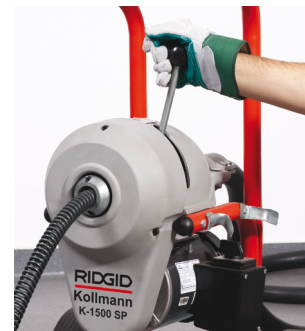
Release handle, cable stops instantly
